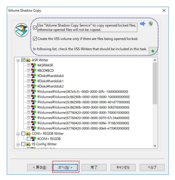
If the task needs to copy the opened/locked files, "Use "Volume Shadow Copy Service" to copy opened files....." option must be checked.
