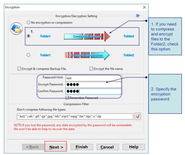
When the encryption option is selected, BestSync compress the file first then used AES 256bit algorithm to encrypt the file.
