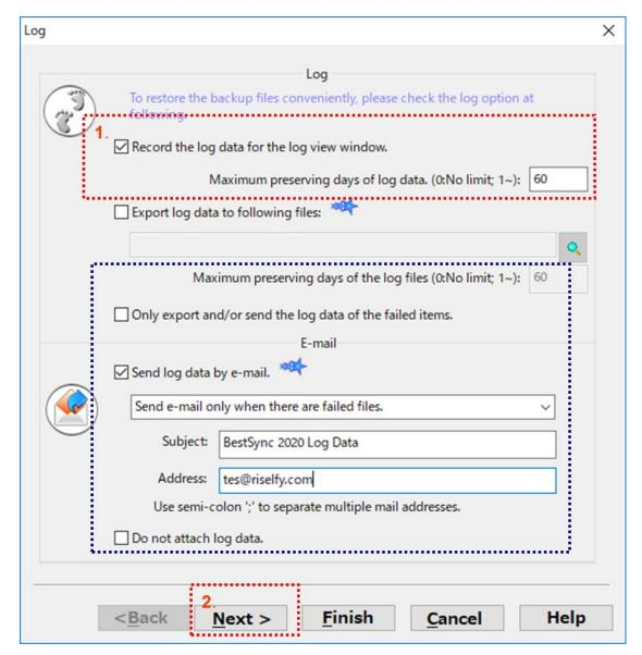
Check the "Record the log data for the log view window" option. This option will record the log data of the synchronization. You can view the log data by the Log View, and if you have setup the "Backup" option in "step 4", you can also restore the backup data conveniently in the Log View.
